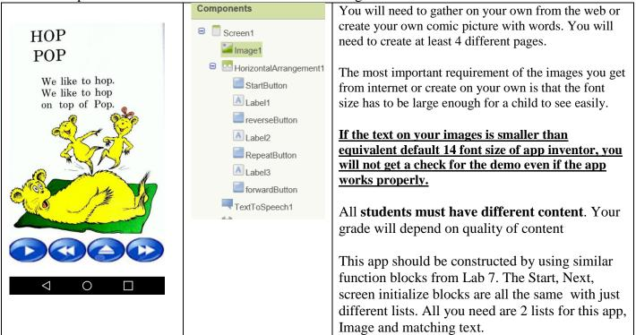
Use Backpack to move similar blocks from Lab 7 to lab 8 and then modify the blocks content to suit the purpose of this simpler app.
